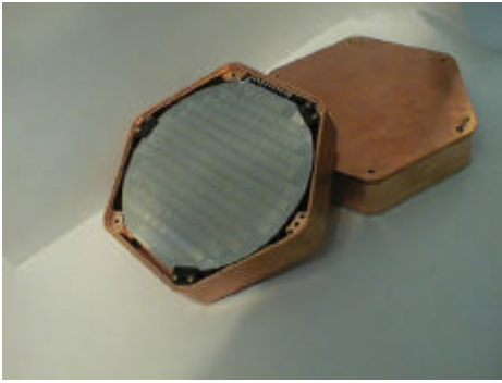
This is a picture of a "ZIP detector." It is an older model that has been used in hopes to detect WIMPS.
